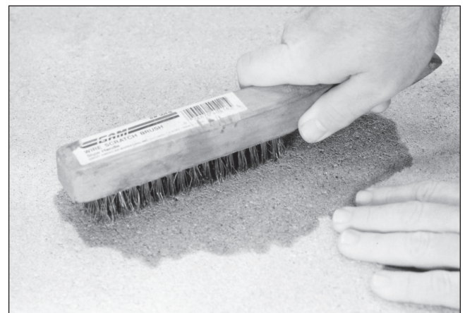
Figure 1 – Conditioning the surface for gage installation.
